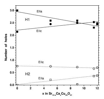
FIG. 7. Hole count per formula unit as derived from renormalized spectral weights in NEXAFS (see text) for  $Sr_{14-x}Ca_xCu_{24}O_{41}$ . Shown are contributions from O 2p orbitals oriented along the a and c axes in chain and ladder units.
