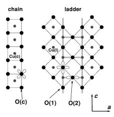
FIG. 1. Structural elements of  $Sr_{14}Cu_{24}O_{41}$ . Shown are chain units consisting of Cu(c) and O(c) sites, and ladder units consisting of Cu(l) and O(1,2) sites, with the "legs" and "rungs" highlighted for one ladder as shaded lines. The chain and ladder layers are stacked alternatingly along the b axis, with Sr sites in between, to form the actual crystal structure.
