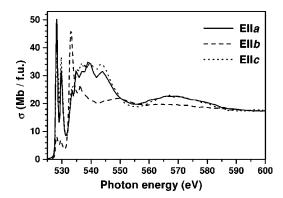
FIG. 2. Polarization-dependent O 1s absorption spectra for  $\operatorname{Sr}_{14}\operatorname{Cu}_{24}\operatorname{O}_{41}$ . For  $\mathbf{E}\|a,c$  two large pre-peaks appear below the main absorption edge at about 535 eV; for  $\mathbf{E}\|b$  these prepeaks are far smaller and a dominant, Sr-related structure appears at the main absorption edge.
