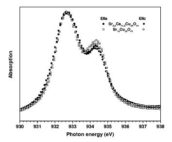
FIG. 6. Polarization-dependent Cu  $2p_{3/2}$  NEXAFS for  $Sr_{14}Cu_{24}O_{41}$  and  $Sr_{2.5}Ca_{11.5}Cu_{24}O_{41}$ , taken in fluorescence yield mode but with no self-absorption correction applied (see text). All spectra are normalized to equal amplitude in the "white line" around 932.5 eV. The ligand-hole peak at about 934 eV provides evidence that  $t_{pd}$  is reduced for high Ca substitution for Sr.
