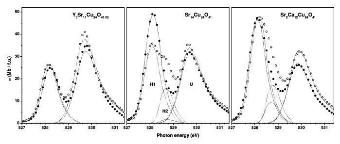
FIG. 4. NEXAFS spectra of  $Y_3Sr_{11}Cu_{24}O_{41}$ ,  $Sr_{14}Cu_{24}O_{41}$ , and  $Sr_2Ca_{12}Cu_{24}O_{41}$  for  $\mathbf{E}\|a$  (filled symbols) and  $\mathbf{E}\|c$  (open symbols) along with the fitted partial distributions corresponding to holes (H1 and H2) and to the upper Hubbard band (U); see text. Spectral weight above 531 eV corresponding to states other than H and U was subtracted (Ref. 32).
